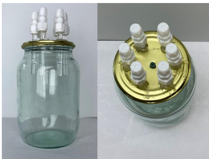
Figure 32 – The 1 L jar with modified caps and six glass capillaries
